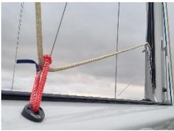
**To minimize the risk of raising the mainsail without removing the boom-cover. We recommend connecting the halyard to the small ANTAL pad-eye mounted on the side of the boom. This can be used to indicate whether the boom-cover is closed.**
