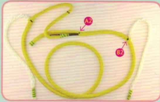
Insert the fid into the cover at A2. Take the cover from the other end and tape it to the fid.
