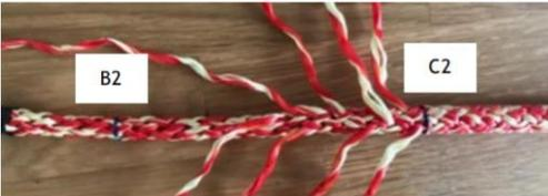
Take the end of the loose cover and stretch it out. When stretched, mark it at 40cm from point A. Let us call this B2. Make another mark, C2, at 12cm from B2. Starting at C2, thin out the cover. Keep in mind that you need to keep the structure of the braid, so take out no more than 8 strands.
